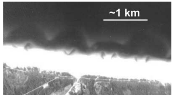
Figure 1. Aerial photograph of a double-barred beach along the Aquitanian Coast revealing the systematic occurrence of two inner-bar rip channels within one outer-bar crescent, suggesting inner-bar variability to be a forced response to outer-bar patterns rather than local free instabilities.
